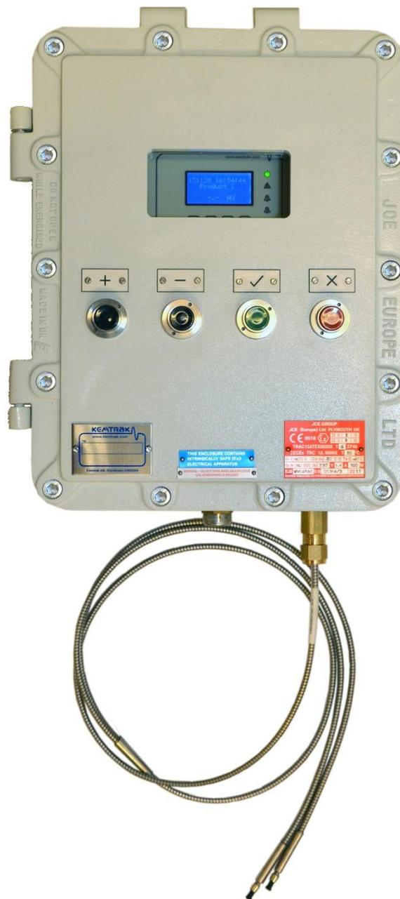
Above: Kemtrak DCP007 industrial photometer housed in an ATEX EExD zone 1 explosion proof enclosure
