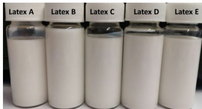
Fig. 3. Samples Latex A, Latex B, Latex C, Latex D and Latex E show a homogeneous particle distribution after 6 days measurement time
