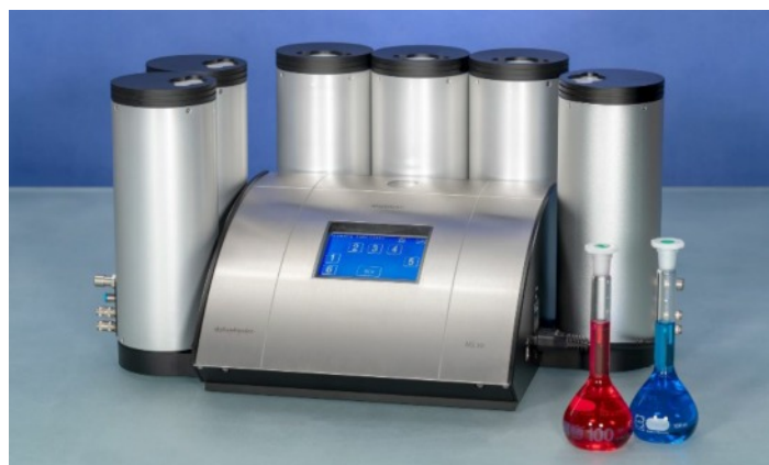
Fig. 2. DataPhysics Instruments stability analysis system MultiScan MS 20 with six independent Scan Towers.
