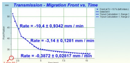
Fig. 7: Migration front vs. time (position 32 mm – 54 mm) of pils beer.
