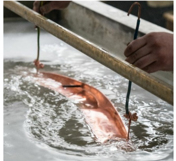
Fig. 1. Example of an electroplating bath.
